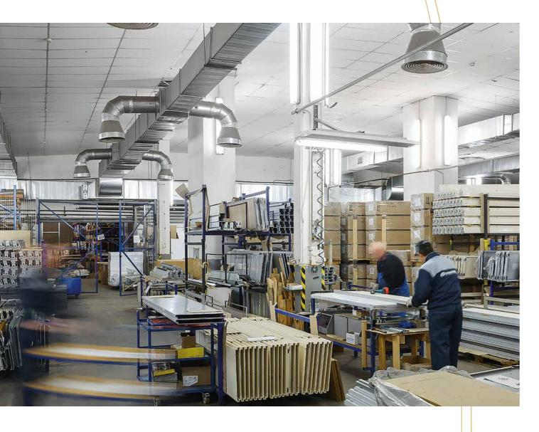
The elevator units are assembled here: fitting the elevator equipment (buffers, overspeed control units, tensioners, steel ropes, etc.), assembling compartment cabins, assembling hoistway door mechanisms, fitting components for installing the guides, assembling cabin and counterweight frames, hoist frame, etc.
